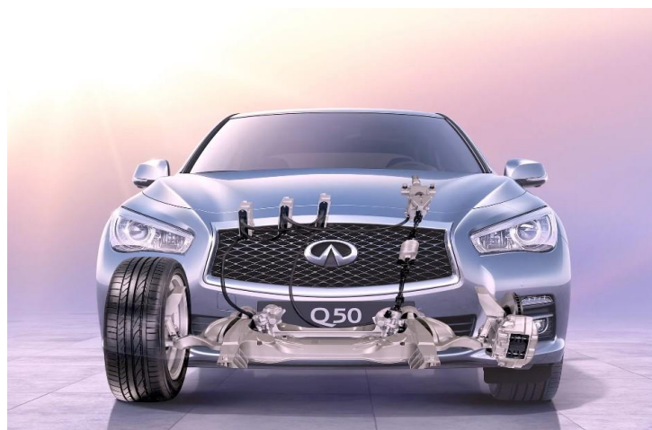
Figure 5: Scheme of the steer-by-wire system of Infiniti.
